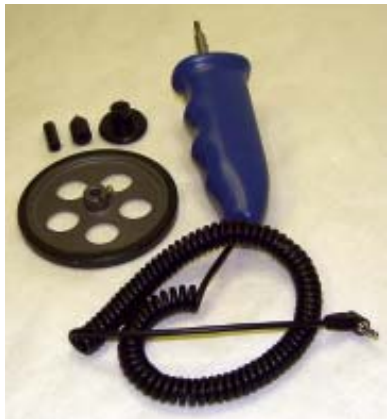
Remote Magnetic Sensor (MT-190-P) Gap 0.25 inches
