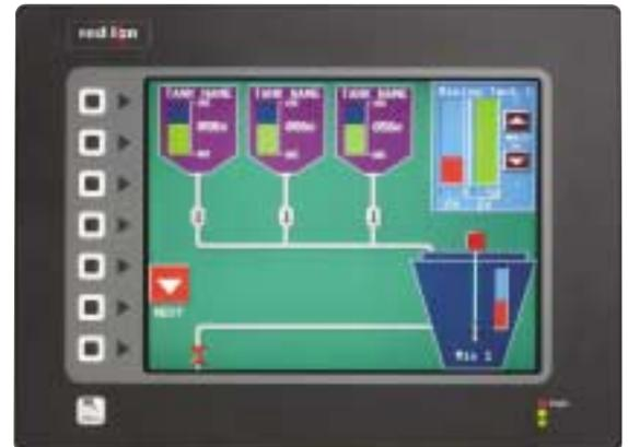
■ The **G310** operator interface touchscreen terminal offers the same features as the G308 in a larger 10.4" active matrix VGA color display size. The G310 includes an eight-key programmable membrane keypad, 3 user-programmable LEDs, and 8MB of on-board Flash. The expansive G10 panel measures 9.50" x 12.83" (241.3 x 325.8 cm) and occupies a depth of only 2.2" (56 cm).
