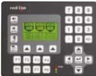
■ The **G303** operator interface terminal offers a 3.2" graphic LCD surrounded by a durable 32-key membrane keypad including five navigation keys, 10+2 numeric keys, 4 dedicated keys, 8 user-legendable keys and 3 soft keys for on-screen menus. Features backlit display, 3 user-programmable LEDs, and 4MB of on-board Flash memory. The compact G303 panel measures 5.85" x 7.45" (148.6 x 189.2 cm), requiring only 2.1" (52 cm) depth.
