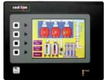
■ The **G306** operator interface touchscreen terminal is perfect for applications that have limited space. With its 5.7" ultra-DSTN quarter VGA display, the G306 offers an easy-to-view display in a smaller package. With its four key programmable keypad, the G306 can utilize pop-up menus to make the most of the limited display size. The G306 measures 7.08" x 8.83" (17.98 x 22.43 cm) and requires a depth of only 2.3" (5.84 cm).
