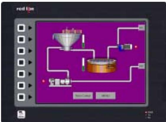
■ The **G310S OUTDOOR** visible operator interface is identical to the standard G310, but offers a super bright 10.4" TFT display that is easily viewable in sunlight. With its special UV resistant overlay and full 0° to 50°C operational temperature range, the G310S is truly designed for the rigors of the outdoors.
